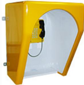
For external or internal use, the T5000 Marine is designed to attain a high level of noise reduction up to 23dB. Manufactured using general-purpose resin mat to BS476 Class 1 fire retardancy, the T5000 Marine is extremely robust and weatherproof. Inside the hood's outer shell is a perforated polypropylene lining that houses 50mm non-hygroscopic acoustic insulation.
